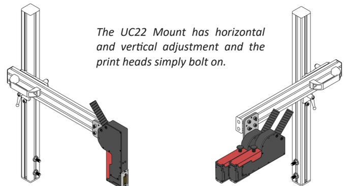
*The UC22 Mount has horizontal and vertical adjustment and the print heads simply bolt on.*
