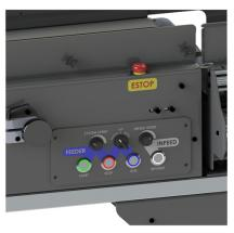
OP Console with integrated reverse for infeed
